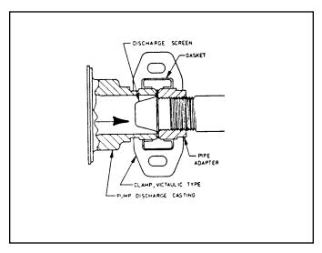
Figure 3.2 Installation of Discharge Screen
